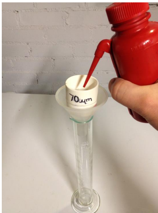
Figure 1. Small diameter sieve on graduated cylinder set up
