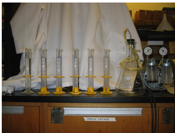
Figure 2. Suggested set up for gravity settling steps
