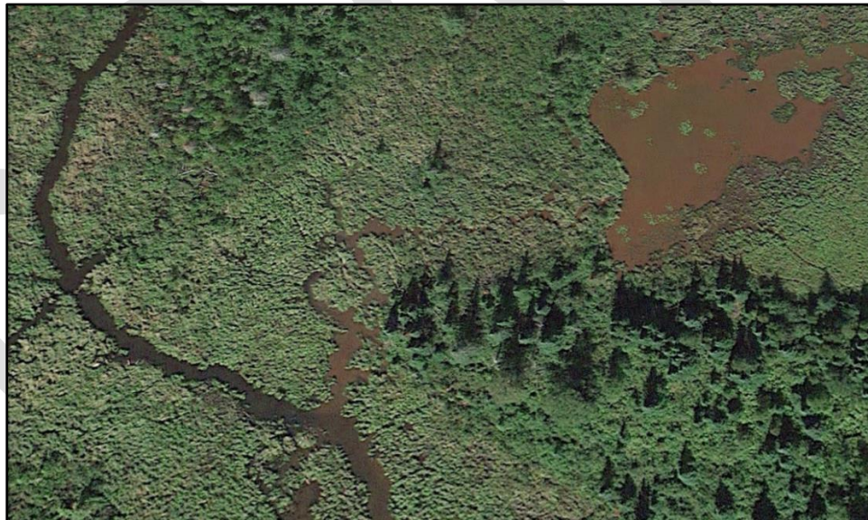
Figure BLANK: Iron precipitate ( \text{Fe}^{3+} ) rust colored water on upper right) forming in tributary stream to Wyman Creek. This particular stream has no upstream mining impacts, which is evidence that natural conditions in the watershed are favorable for the formation of \text{Fe}^{3+} .
