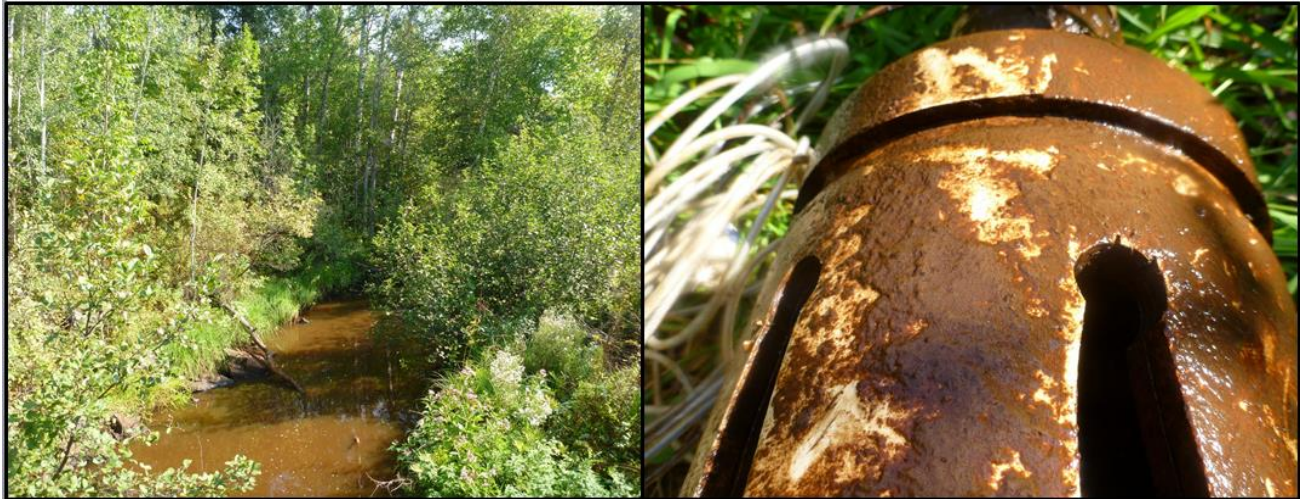
Figure BLANK: Iron precipitate observed at Wyman Creek biological monitoring station 81LS008 on 9/12/2012. The photo on right shows accumulation of precipitate on a barrel that was deployed in the stream for one week.
