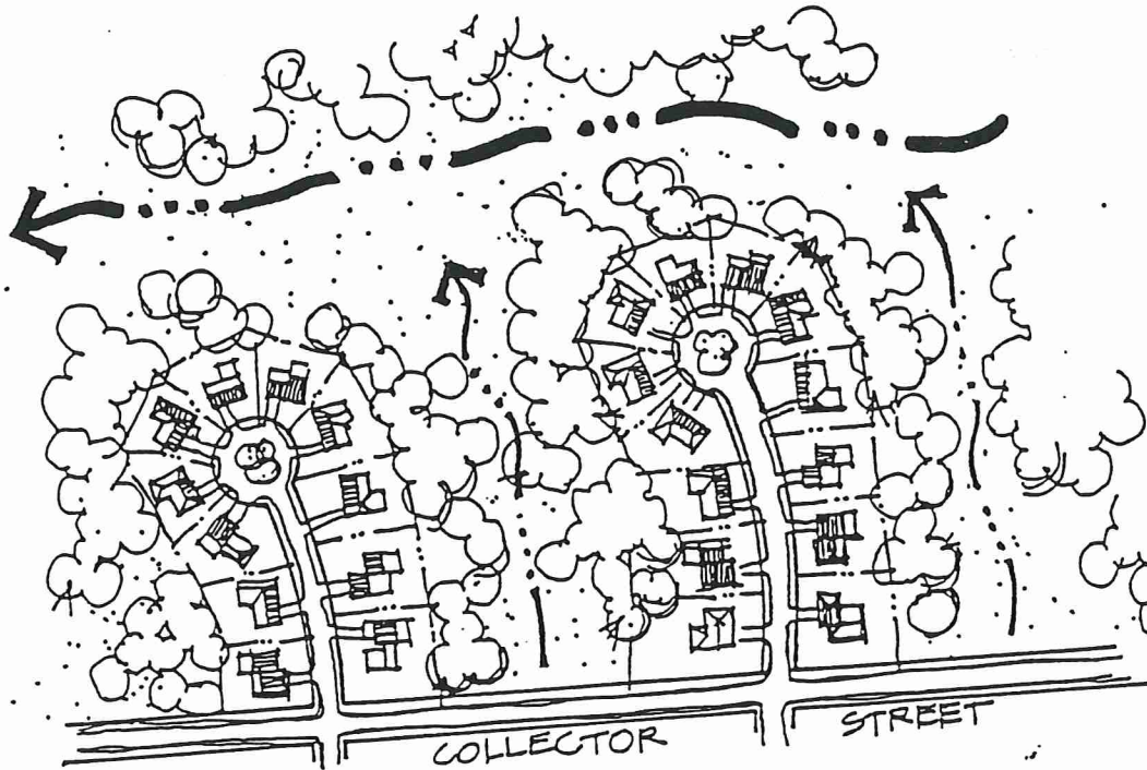
FIGURE VI-3 Use sensitive areas such as natural drainage areas to form boundaries or buffer zones between clusters of housing.
