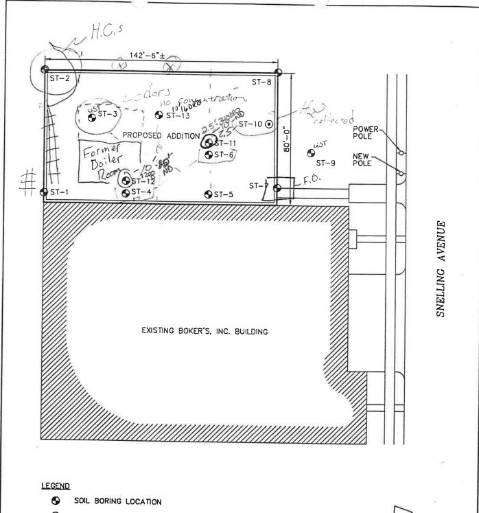
HYDROPUNCH WATER SAMPLE/SOIL BORING LOCATION
