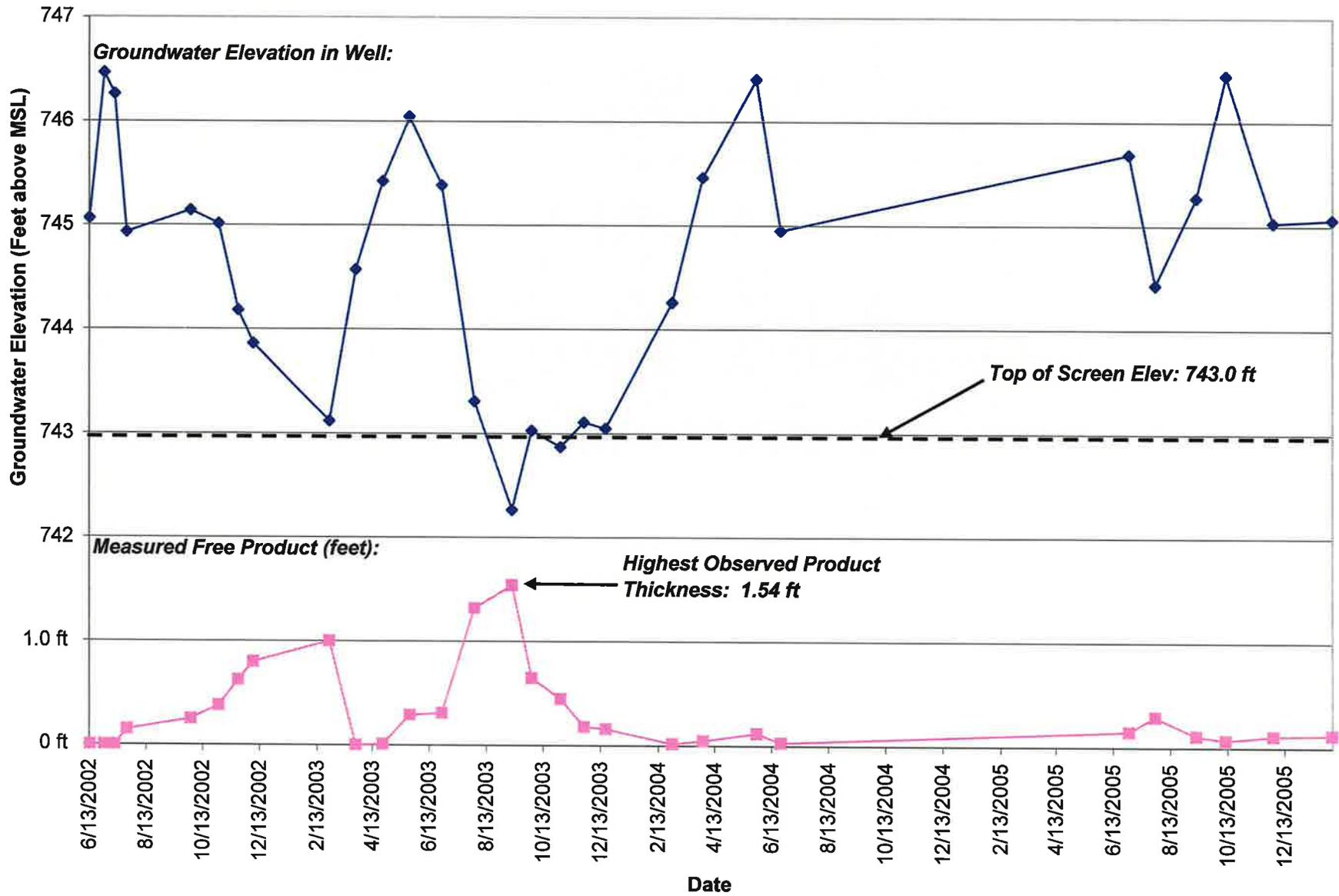
**Figure 8: MW-2 Hydrograph
