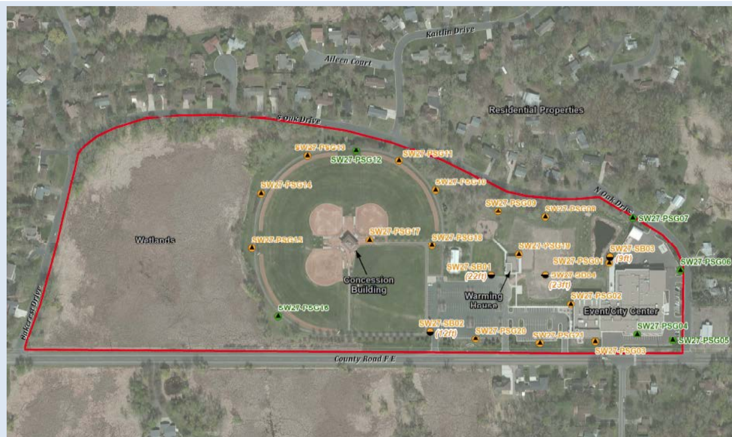
Map of the former Vadnais Heights landfill showing locations of soil borings and permanent soil gas sampling points.
