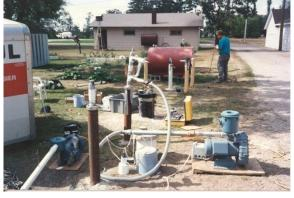
enhanced free-product recovery extracts light non aqueous phase liquids (LNAPLs) from the capillary fringe and the water table.
