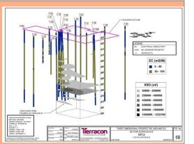
probes were advanced to depths of 55 to 66 feet below ground. In addition, some of the MIP probes were advanced at angles to obtain data from below the on-site building. The MIP data provided additional information pertaining to the TCE source mass and distribution of TCE in the subsurface which was observed to coincide with the bottom of a silty soil layer located at approximately 45 feet.
