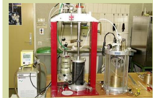
For the SLRIDT Superfund site in Duluth, Barr conducted extensive bench testing, including this seepage-induced consolidation test to determine the consolidation properties of watery sediments not testable with conventional equipment.
