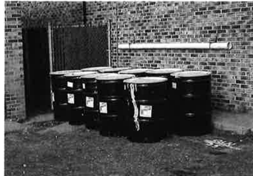
Drums containing soil cuttings
