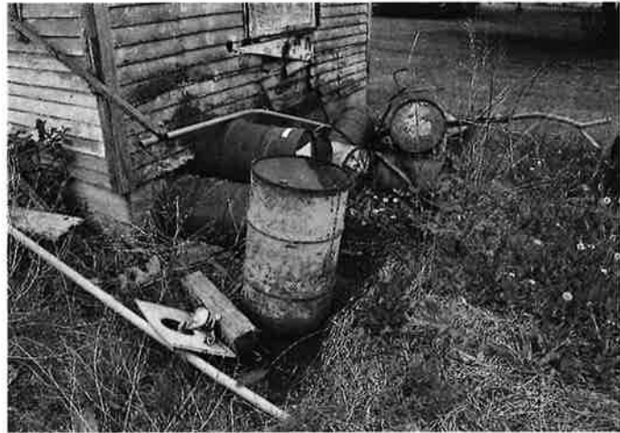
Drums in poor condition, releasing oil to soil surface
