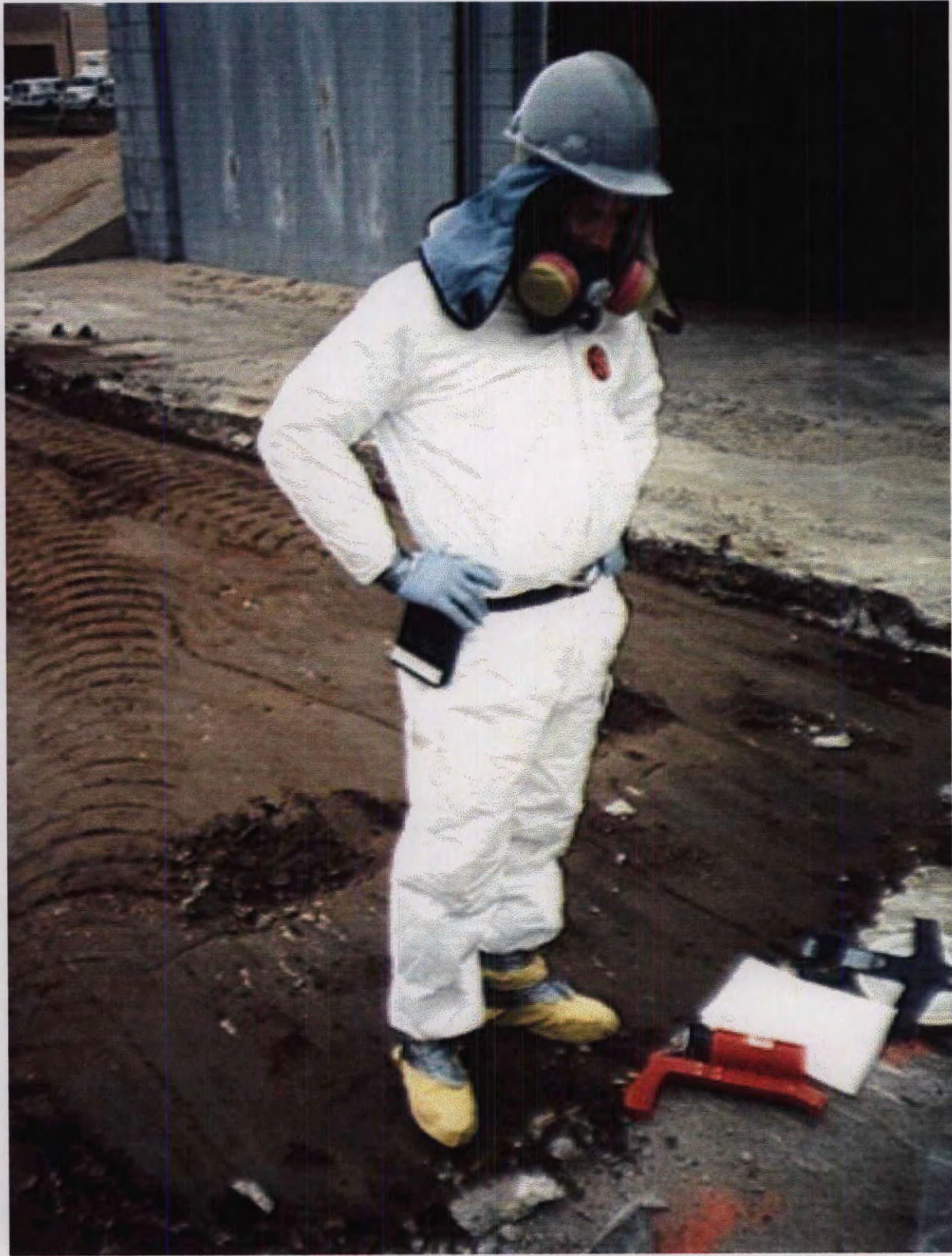
Photo 9 Personnel Particulate Sampler and Other Personnel Protective Equipment
