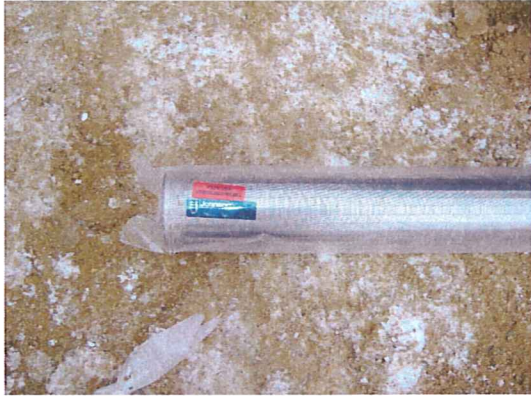
Feb. 5 thru 12, 2008 - DPE and monitoring well screen
