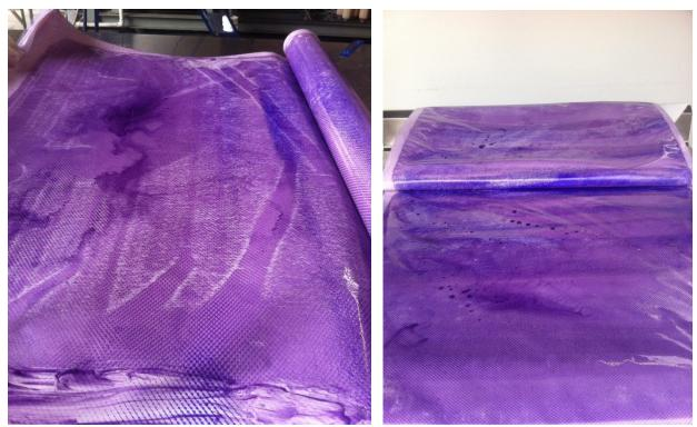
110322229 (6-3) – Dye coating the feed side of the membrane surface
