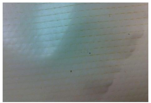
Element 'O' – Example of Element Fouling and Particulate Matter
