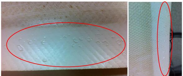
110322090 (6-2) – "Bubbling" within the membrane glue line (left, right).
