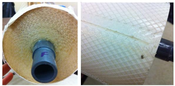
Element 'O' – Feed(L) and Concentrate(R) Side of Membrane with ATD Removed
