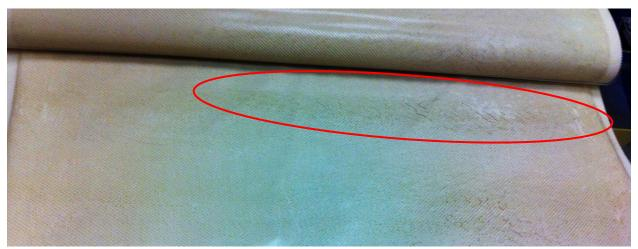
110322090 (6-2) – Heaviest foulant accumulation near the permeate core tube.
