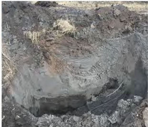
Ash sidewall at FD-TT-03
