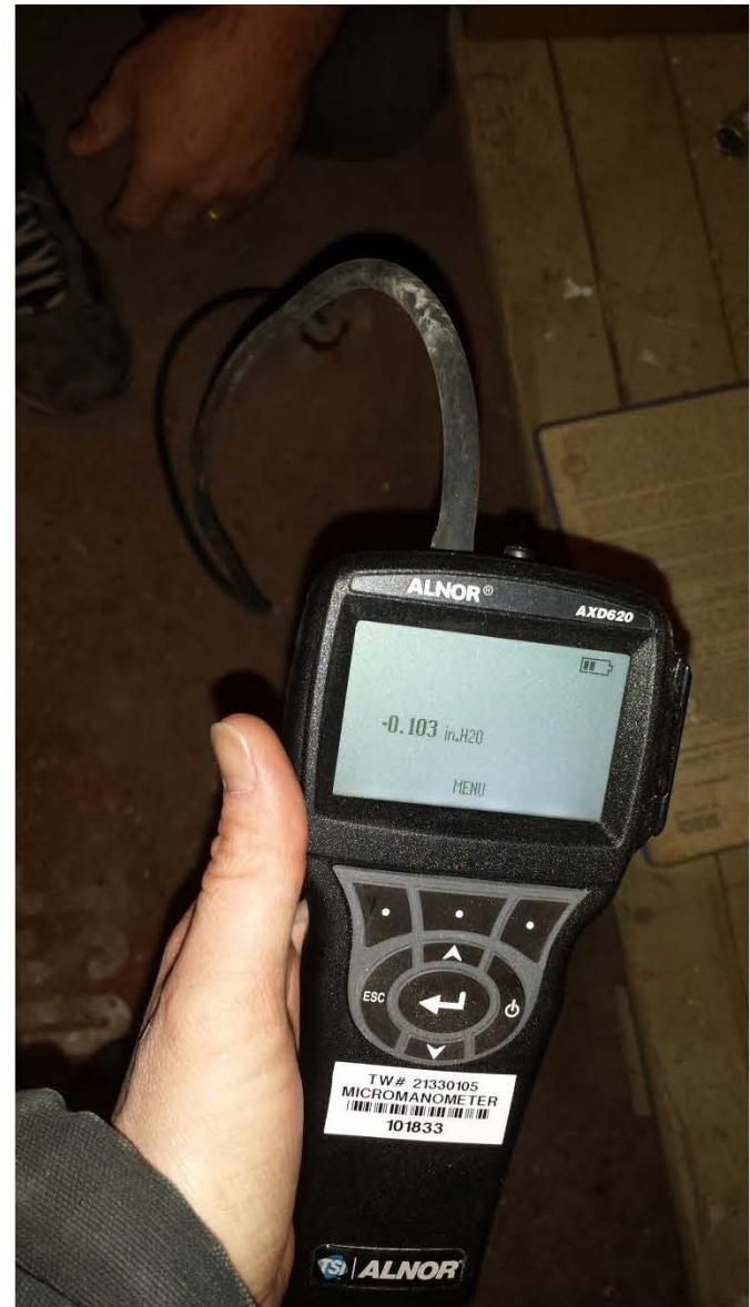
Photo 24: View of final mitigation system test point readings: TP-04 reading.
